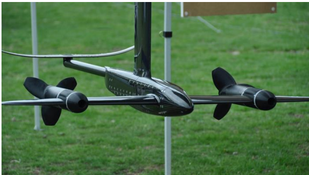
Figure 7: KTH test rig for new hydrofoiling concept with patented electric motor pods mounted on the wings and a unique roll stabilization configuration based on a mast rudder.
